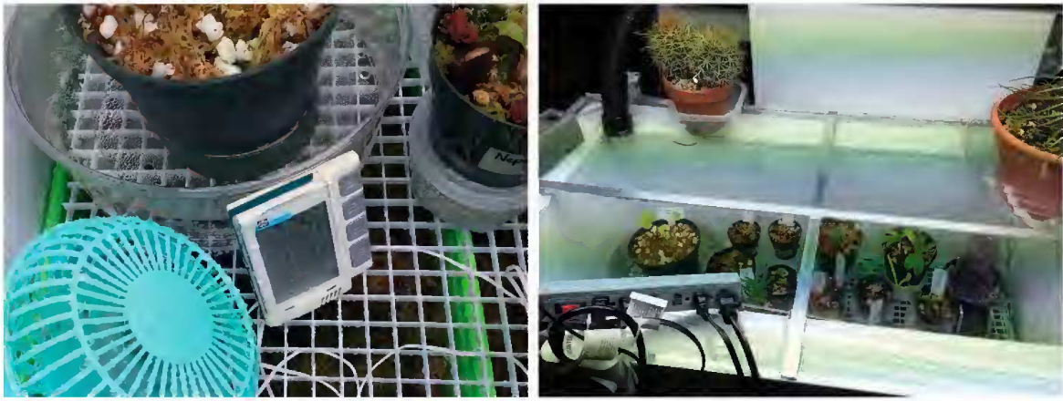
Figure 3: The completed chamber. A $4 USB fan circulates the air and prevents moisture accumulating on the foliage.
